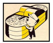
You've all heard the expression "beaten to a pulp." Beating and refining is the next step. The pulp, which is suspended in water, is fed through a machine with a rolling drum and knives that pull apart the fibers. The ends of the fibers become frayed and this helps to make the fibers felt together after the water is drained. This helps to form a uniform sheet of paper. The beating process takes several hours and during this time, the color and sizing materials are added.
