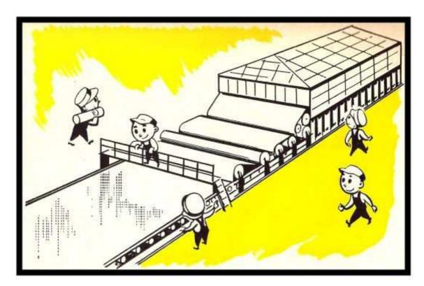
Paper that comes from the dryers is not smooth enough for most purposes. A finish must be applied by running the sheet a specified number of times through a series of polished steel rollers and by the amount of weight or pressure applied. The finished paper is wound onto large rolls that are either cut into smaller rolls or sheets and then it is packaged for distribution.
